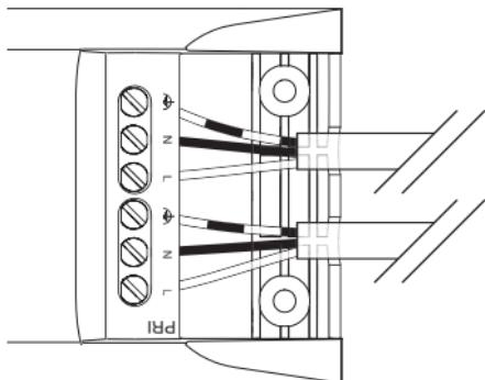
Durchverdrahtung / Through-wiring /
