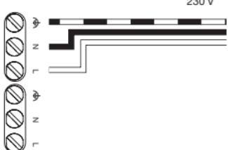
Durchverdrahtung / Through-wiring /
