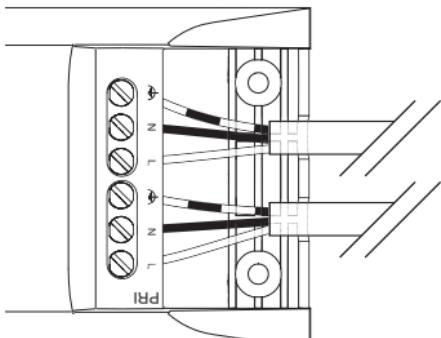
Durchverdrahtung / Through-wiring /
