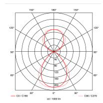
Sento E (satinised glass / lense) reflector head for diffuse light in one and directed light in the other direction
