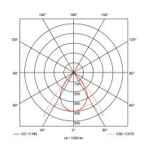
Sento C (cover / lense) reflector head for directed light in one direction
