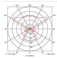
**Divo E** reflector head for light with narrow radiation to one and wide radiation to the other side
