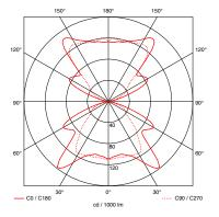
reflector head for light with narrow radiation
