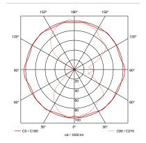
**Divo A**Reflector head for spherical light, radial distribution
