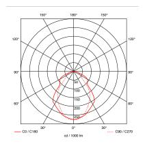
reflector head for light with narrow radiation to one side
