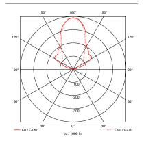
**Divo B** reflector head for light with wide radiation to one side
