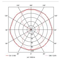
**Divo A**Reflector head for light with open luminaire and radial distribution
