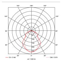
reflector head for light with narrow radiation to one side
