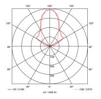
**Divo B** reflector head for light with wide radiation to
