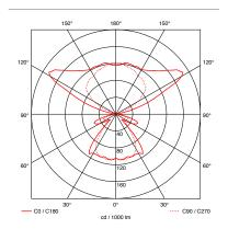
reflector head for light with wide radiation to one and narrow radiation to the other side
