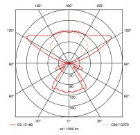
reflector head for light with wide radiation to one and narrow radiation to the other side
