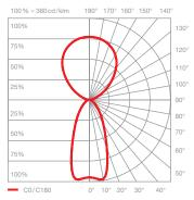
room (narrow) concentrated light downwards, beam angle approx. 50°, diffuse upwards
