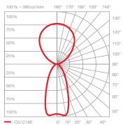
room (narrow) concentrated light downwards, beam angle approx. 50°, diffuse upwards
