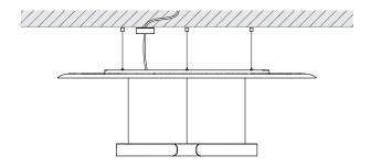
${\bf Trac\ adapter}$  for 3-phase Erco-, Zumtobel- or Eutrac-bus-bar, connection to 230 VAC/50 Hz mains voltage (DALI optional only Eutrac).
