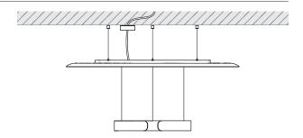
$\mbox{Trac}$  adapter for 3-phase Erco-, Zumtobel- or Eutrac-bus-bar, connection to 230 V AC / 50 Hz mains voltage (DALI optional only Eutrac).
