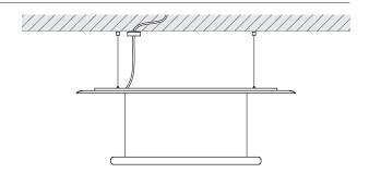
${\bf Trac\ adapter}$  for 3-phase Erco-, Zumtobel- or Eutrac-bus-bar, connection to 230 VAC/50 Hz mains voltage (DALI optional only Eutrac).
